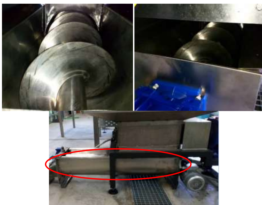
Picture 3. Screw placed after the shredder and before the pump
