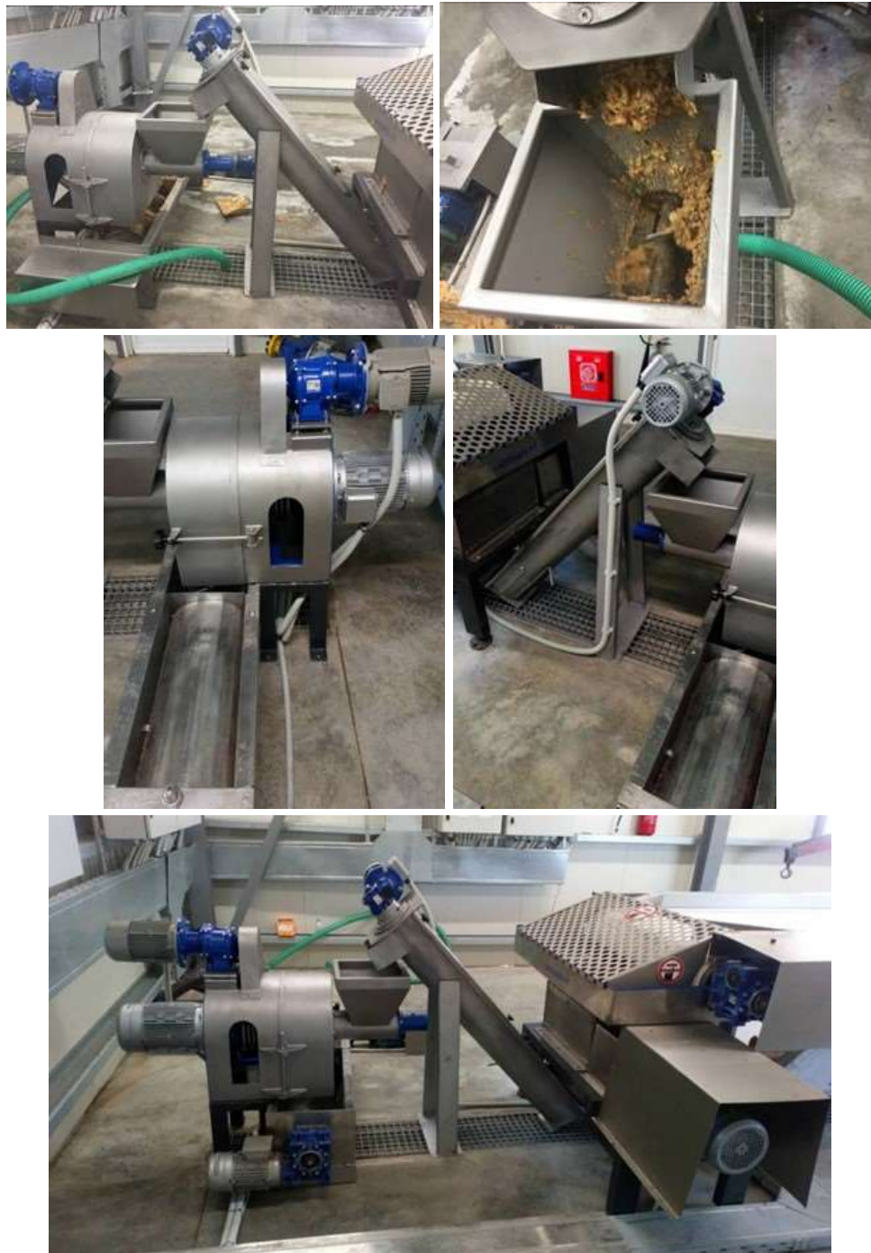
Picture 7. The pulverizer connected after the shredder
