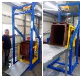
Picture 12. Hydraulic lifting system
